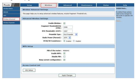
**Enabled Wireless**: Enabled or Disabled wireless function
