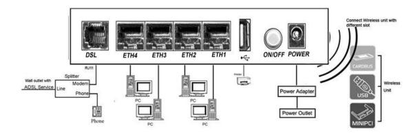
Notes: Without the splitter and certain situation, transient noise from telephone can interfere with the operation of the Router, and the Router may introduce noise to the telephone line. To prevent this from happening, a small external splitter must be connected to each telephone.
