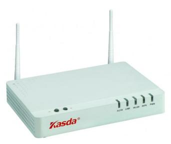
This device is an EPON ONU device. As compared to other broadband access technologies such as xDSL and cable modem, Passive Optical Network (PON) technology offers some compelling advantages, including a long-term life expectancy of the fiber infrastructure, lower operating costs through the reduction of "active" components, support for greater distances between equipment nodes, and most importantly, much greater bandwidth.
