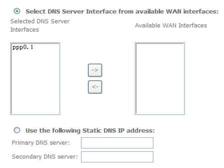
11. Make sure that the settings below match the settings provided by your ISP. Click on the **Apply/Save** button to save your configurations and reboot the ADSL router.
