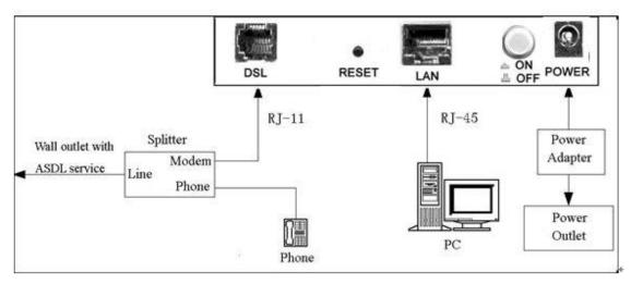
Notes: Without the splitter and certain situation, transient noise from telephone can interfere with the operation of the ADSL router, and the ADSL router may introduce noise to the telephone line. To prevent this from happening, a small external splitter must be connected to each telephone.
