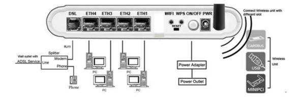
Notes: Without the splitter and certain situation, transient noise from telephone can interfere with the operation of the Router, and the Router may introduce noise to the telephone line. To prevent this from happening, a small external splitter must be connected to each telephone.
