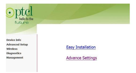
We can select Easy Installation or advanced Settings mode to setup KW5815.the Easy Installation will guide us for a basic setting, and the advanced Settings will guide us to home page for more detailed setup.
