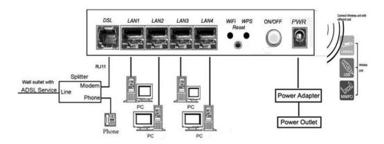
Notes: Without the splitter and certain situation, transient noise from telephone can interfere with the operation of the Router, and the Router may introduce noise to the telephone line. To prevent this from happening, a small external splitter must be connected to each telephone.
