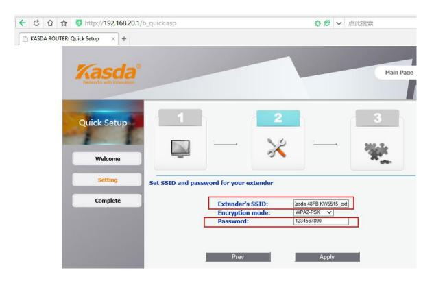
**STEP 7:** After the settings are 100% saved and applied, the connection between laptop and Extender will be disconnected automatically, you need to reconnect to the Extender's new **WiFi network name** with new **WiFi password**, as showed in below screen.
